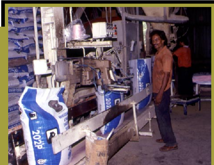
Sacking-off process at the Port Klang Feedmill factory.
